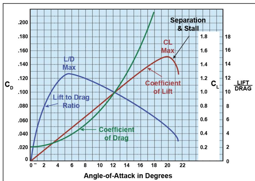
Figure 2. Lift/drag curve.
