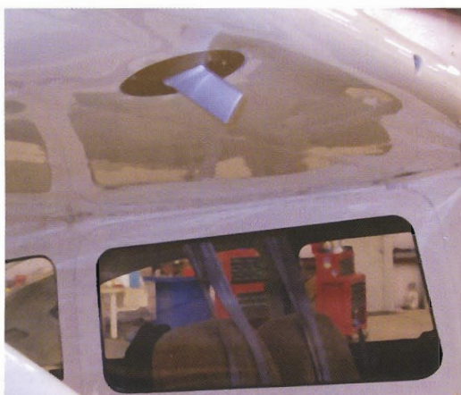
The probe was installed here to minimize the "head-knocker" hazard.
