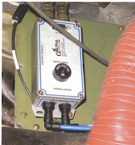
Above, left: The original models of the Alpha Systems AOAs included straightforward dial-type displays. Above, right: The control module is mounted near a duct.
