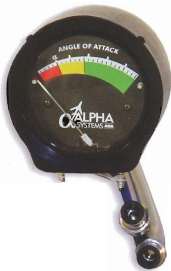
Above, left: The original models of the Alpha Systems AOAs included straightforward dial-type displays. Above, right: The control module is mounted near a duct.
