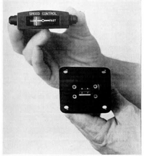
The simplest, cheapest angle-of-attack indicator yet manufactured: For \$300, you get a transmitter (bottom), which replaces the stall-warning vane in the leading edge of the wing, and an indicator (top) for mounting in the cockpit.
